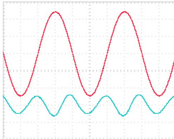
DISTORTION @ 3 WATTS / 4 OHM
