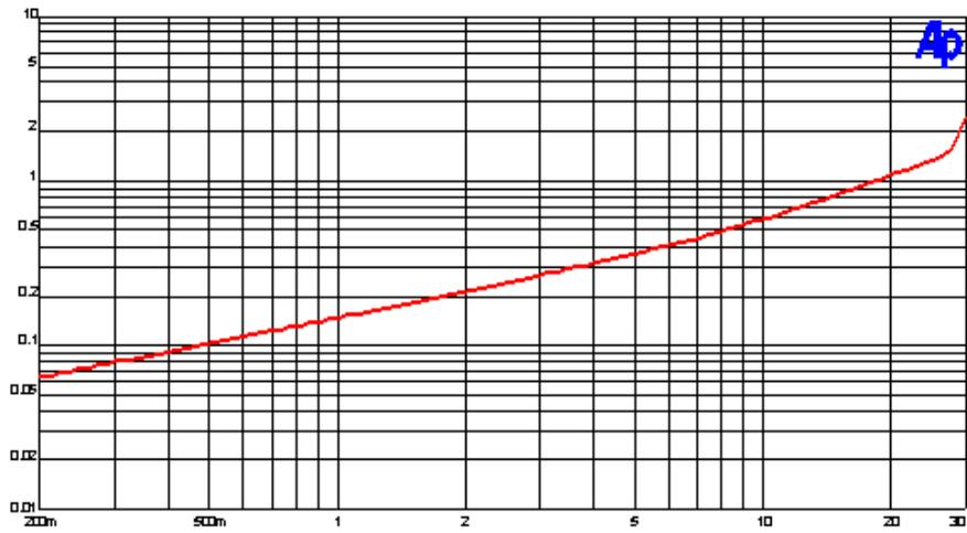
SIT-3 DISTORTION VS OUTPUT WATTS @ 4 OHMS
