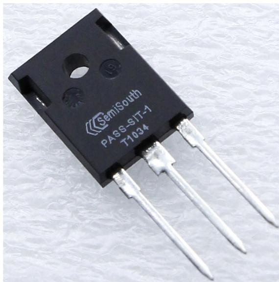
Unfortunately, there was only one production run of this transistor, commissioned by First Watt and made by SemiSouth, now defunct. Most of the SIT parts were used in the first two amplifier models, but nearly half were held for service and also this new design.
